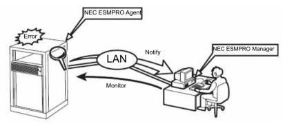
When a failing module in the server is to be replaced, NEC ESMPRO Manager enables logical module disconnection from the server and logical installation after module replacement.
